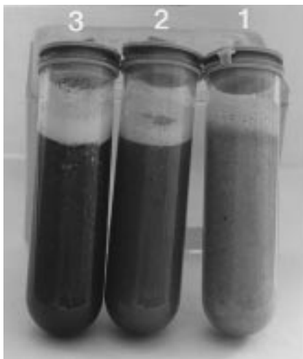
Figure 6. Effect of the absence/presence of 2-OH-P- \beta -CDs in banana pulp extract. The reaction medium at room temperature contained 50 g of banana pulp and 75 mL of 100 mM phosphate buffer (pH 7.3) (tube 1), 50 g of banana pulp and 75 mL of 10 mM 2-OH-P- \beta -CDs in 100 mM phosphate buffer (pH 7.3) (tube 2), or 50 g of banana pulp and 75 mL of 100 mM 2-OH-P- \beta -CDs in 100 mM phosphate buffer (pH 7.3) (tube 3). The pictures were taken 30 min after homogenization.
